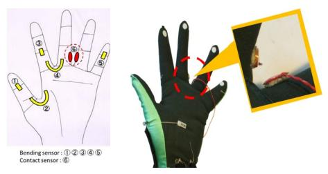
Figure 3. Sensor Layout(left) and the prototype(right).
