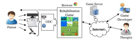
Figure 1. Scheme of the Web-based virtual rehabilitation system.
