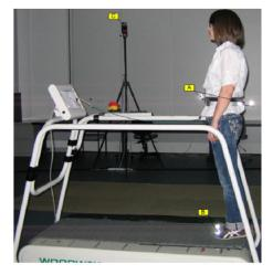
**Figure 2**. A participant using the RTSCA. A: pelvis cluster – a sprung loaded frame with 3point contact to calculate the origin of the pelvis segment; B: markers on feet; C: one of the eight motion capture cameras used.
