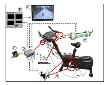
**Figure 1.** Virtual Reality Augmented Cycling Kit (VRACK): A: Sensorized handle bars, B: Sensorized pedals, C: Heart Rate sensor and monitor D: Controller E: Power source F: Practitioner interface (where the target heart rate is set) G: Virtual Environment.
