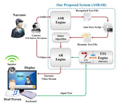
Figure 2. The ASRAR system structure.
