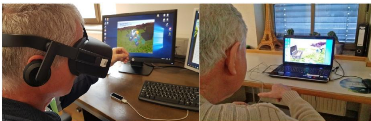
Figure 1. LEFT: Left handed participant practising pinch and place cubes in 3D VE (Oculus Rift CV1). The hand motion is tracked by the small camera on the table. RIGHT: Right handed participant is practising the task on the 15.2" laptop.
