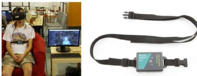
Figure 2. Participant in process of training with presented virtual reality application in interaction with breath bio-feedback and the photograph of the Vernier respiration belt.
