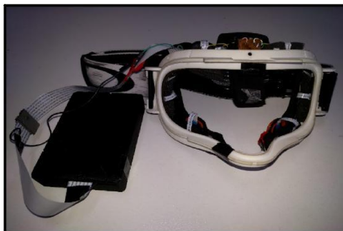
Figure 3. Prototype EMG goggles - Oculus VR headset interface enabling multichannel EMG sensing of multiple facial expressions
