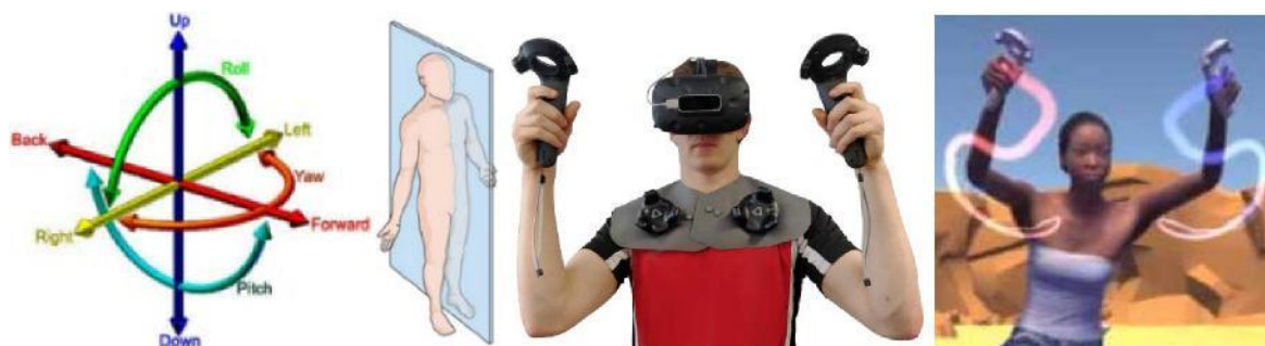
Figure 1. a) 6 DoF and Sagittal Mirror plane b) Mirror VR trackers c) Mirror Mode-C in-game with visual trails
