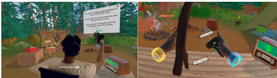
Figure 2. (a) Third person view of VR environment showing unaffected right limb driving a mirrored virtual affected left limb, (b) First person view of reach-and-grasp task and controller instructions.
