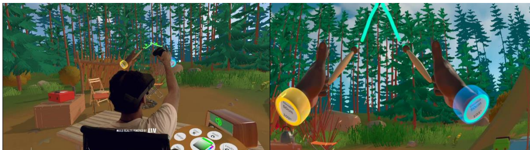
Figure 4. (a) Third person view of VR environment showing the unaffected right limb driving a mirrored virtual affected left limb to draw, (b) First person view showing symmetrical drawing.
