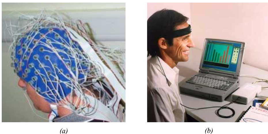
Figure 1. (a) A person's brain activity being measured through EEG signals, and (b) The Cyberlink Mindmouse
