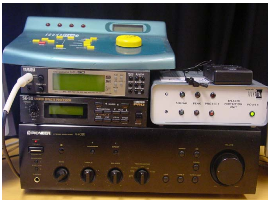
Figure 2 (left) Soundbeam control unit (upper left), stereo sound module and stereo effect processing unit (left middle), speaker protection unit for vibroacoustic soundbox 6 (white) with wireless microphone upon it. All rest upon the main system stereo amplifier
