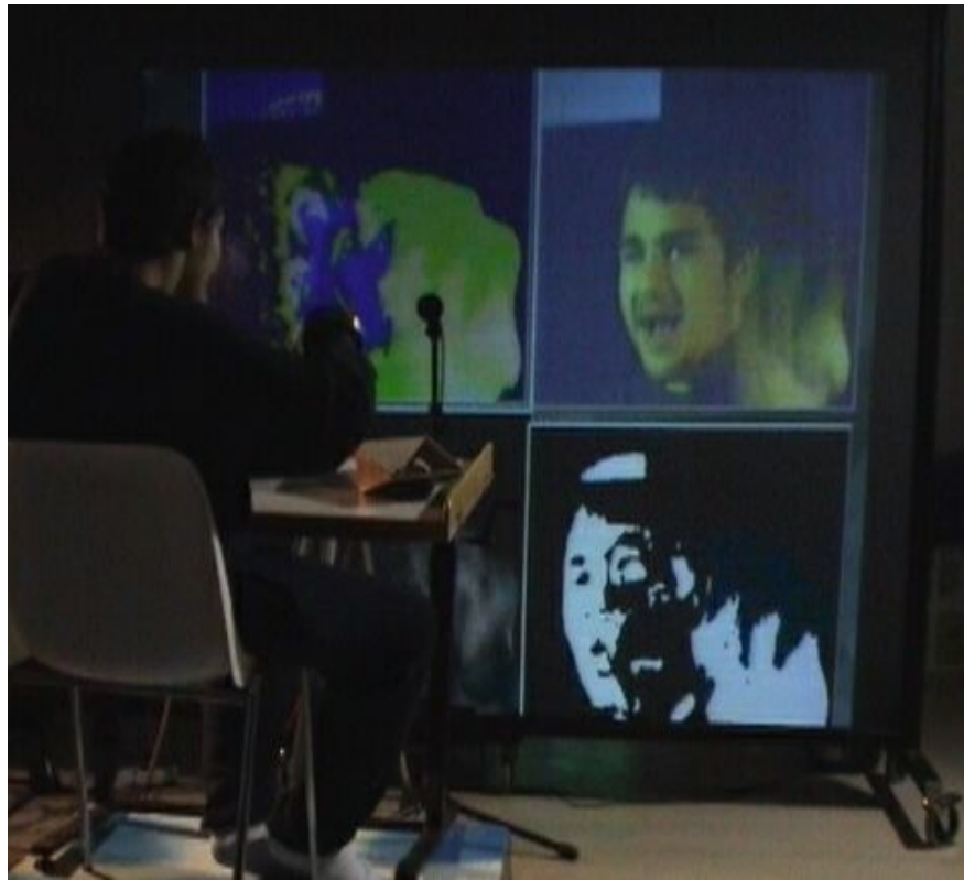
Figure 3 Rasmus sitting upon a chair on the vibroacoustic soundbox which enables him to feel the sounds he generates from his movement in the Soundbeam sensor whilst creating video and sound effects with head, hands and utterances
