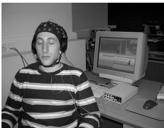
Figure 3. The BCMI mixer system uses an ordinary PC, affordable EEG equipment with serial or USB connection and off-the-shelf software, making it user-friendly and easy to operate.
