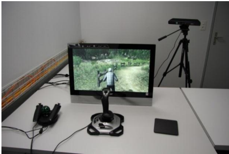
Figure 3. First Study experimental Setup (from left to right: the Razer Hydra, the Joystick, the Touchpad and the Kinect).
