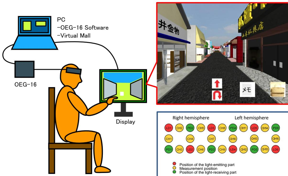
Figure 1. Experimental system with VST-R screen and fNIRS channel arrangement on the forehead.
