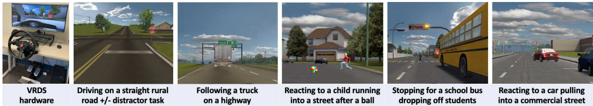
Figure 1 Virtual reality driving simulator (VRDS) equipment setup and driving scenarios.
